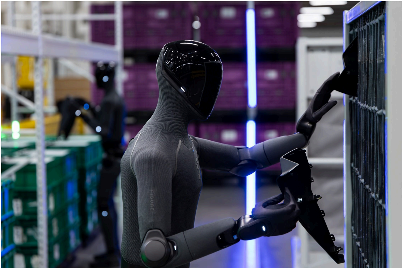
A Figure humanoid moves sheet-metal parts on BMW's Spartanburg line during its eleven-month, 1,250-hour deployment — one of the best-documented cases of sustained humanoid labor anywhere in the industry. Credit: Figure AI/BMW Group
